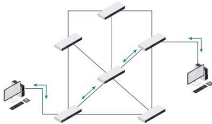
Circuit switched networks provide a dedicated path between nodes. (Image © 123RF.com.)
