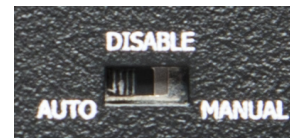
Figure 11-7: SDP Backup Radio Control
