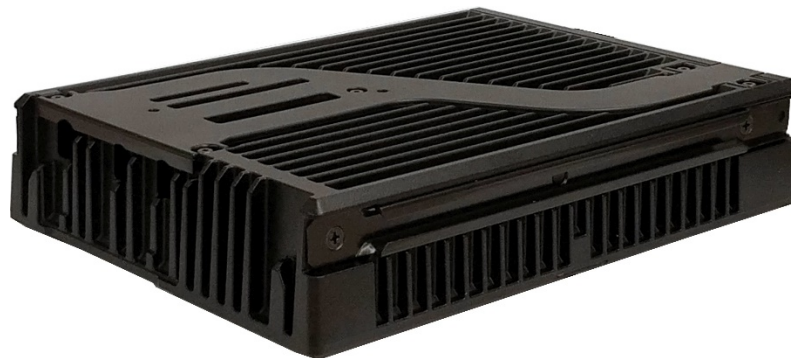
Figure 3-1: Vehicle Communications Hub (VCH)
