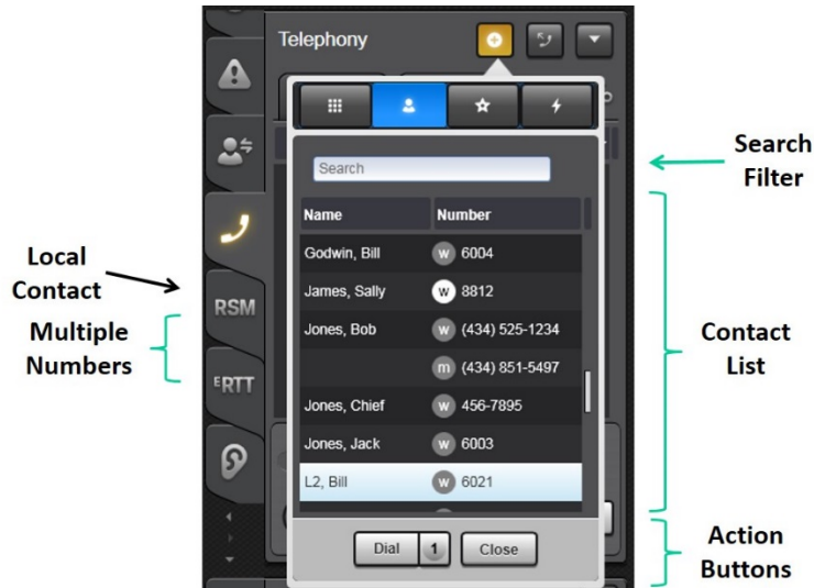
Figure 3-49: Typical Contact View
