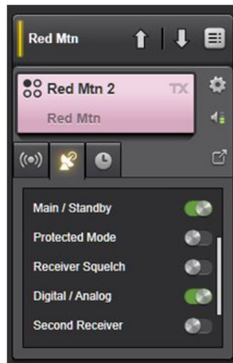
Figure 7-14: Base Station Module in Standby
